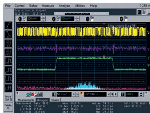
Figure 6. The EZJIT jitter analysis package serves as a powerful jitter debug tool by providing users an integrated and time-correlated view of the signals under test and the jitter measurements.
