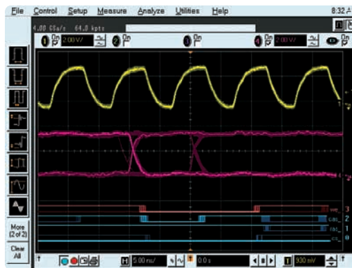
Figure 2. This six-channel measurement wouldn't be possible on a traditional DSO. A mixed-signal oscilloscope, however, enables the scope to trigger on a data “write” with RAS, CAS, WE, CS, and CLK using the 16 logic timing channels. The 4 scope channels are then freed up to evaluate signal integrity. The MSO used for this measurement is the 1 GHz Agilent 54832D.
